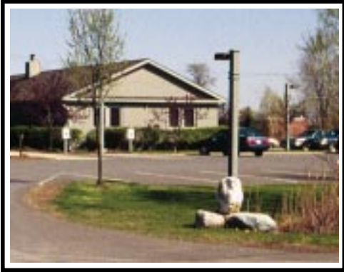
▲ This shielded lamp directs light downward.
